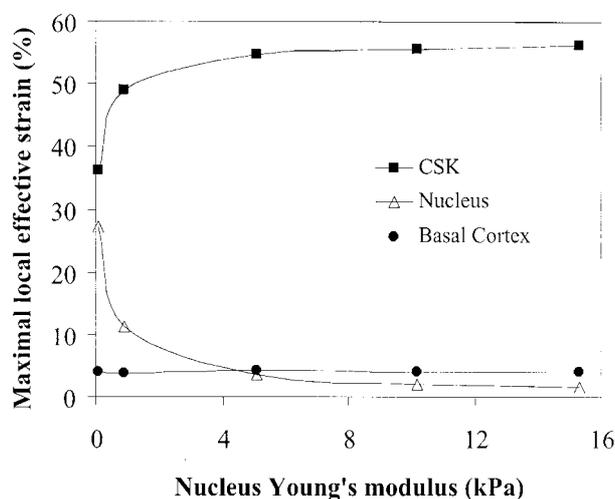
**Figure 8.** Influence of the nucleus stiffness on the amplitude of the maximal local effective strain in the different cell components. In all the simulations, the locations of the maximal effective strains are those indicated on Figure 4. These numerical results are obtained when a rotation of  $25^\circ$  is imposed on the two beads. All computations have been performed with the Std set of parameters except for the parameter under study, i.e. the nucleus Young's modulus.
