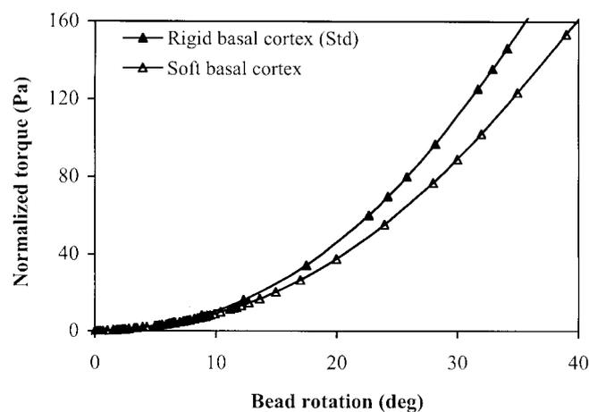
**Figure 10.** Influence of basal cortex stiffness on the hyperelastic torque-bead rotation response. The “Rigid basal cortex” curve is the control simulation obtained with the Std set of parameters (Table 1) with basal cortex Young's modulus  $6a_{1b} = 900$  Pa. The “Soft basal cortex” curve is obtained with the same parameters, except for the basal cortex Young's modulus now equals to 12 Pa.
