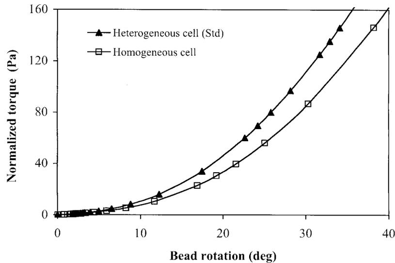
**Figure 3.** Influence of the nucleus stiffness on the mechanical torque-bead rotation response. The Heterogeneous cell curve is the control simulation obtained with the Std set of parameters defined in Table 1. The Homogeneous cell curve is obtained when considering that the cell nucleus and CSK have the same elastic properties. Normalized torque values are obtained by dividing the applied torque  $T$  by the bead volume  $V_b$ .
