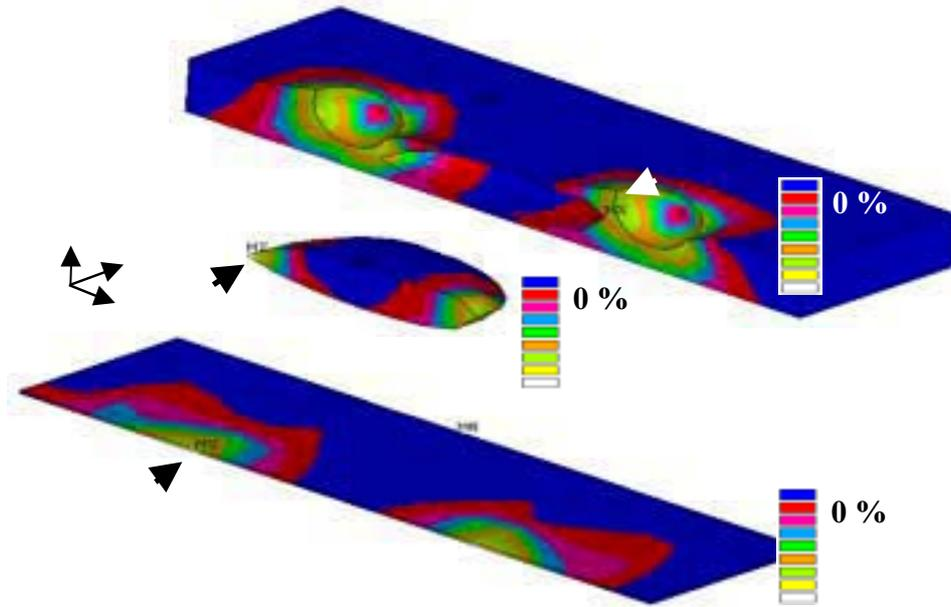
**Figure 5.** Legend as in Figure 4, except that the elastic properties of the nucleus are now those of the CSK. The  $25^\circ$  imposed rotation of the two beads induces a mean bead translation  $\Delta_x$  of  $0.54 \mu\text{m}$ . The resulting normalized mean torque is 56 Pa. Arrows indicate the maximum effective strain locations in each cell constituent.
