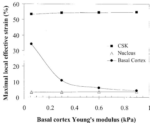
**Figure 9.** Influence of the basal cortex stiffness on the amplitude of the maximal local effective strain in the different cell components. In all the simulations, the locations of the maximal effective strains are those indicated on Figure 4. These numerical results are obtained when a rotation of  $25^\circ$  is imposed on the two beads. All computations have been performed with the Std set of parameters except for the parameter under study, i.e. the basal cortex Young's modulus.
