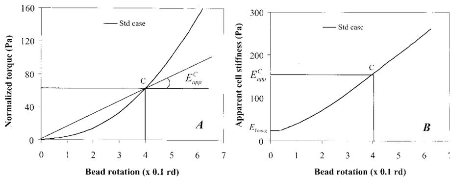
**Figure 7.** Simulated nonlinear elastic response of the adherent epithelial cells obtained with the Std set of parameters. A) Normalized torque-bead rotation response. The apparent cell stiffness  $E_{app}^C$  at a point C of the response curve is defined as the slope of the straight line OC. The torque  $T$  is normalized by the bead volume  $V_b$ . B) Associated variation of the apparent cell stiffness  $E_{app}^C$  for increasing bead rotation derived from Figure 6A.
