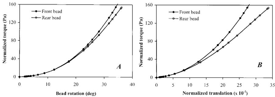
**Figure 6.** Mechanical response of the front and rear beads simulated with the Std set parameters. A) Nonlinear torque-bead rotation response curves. B) Nonlinear mechanical torque-bead translation response curves. The bead translation  $\Delta_x$  is normalized by the bead radius  $R$ .
